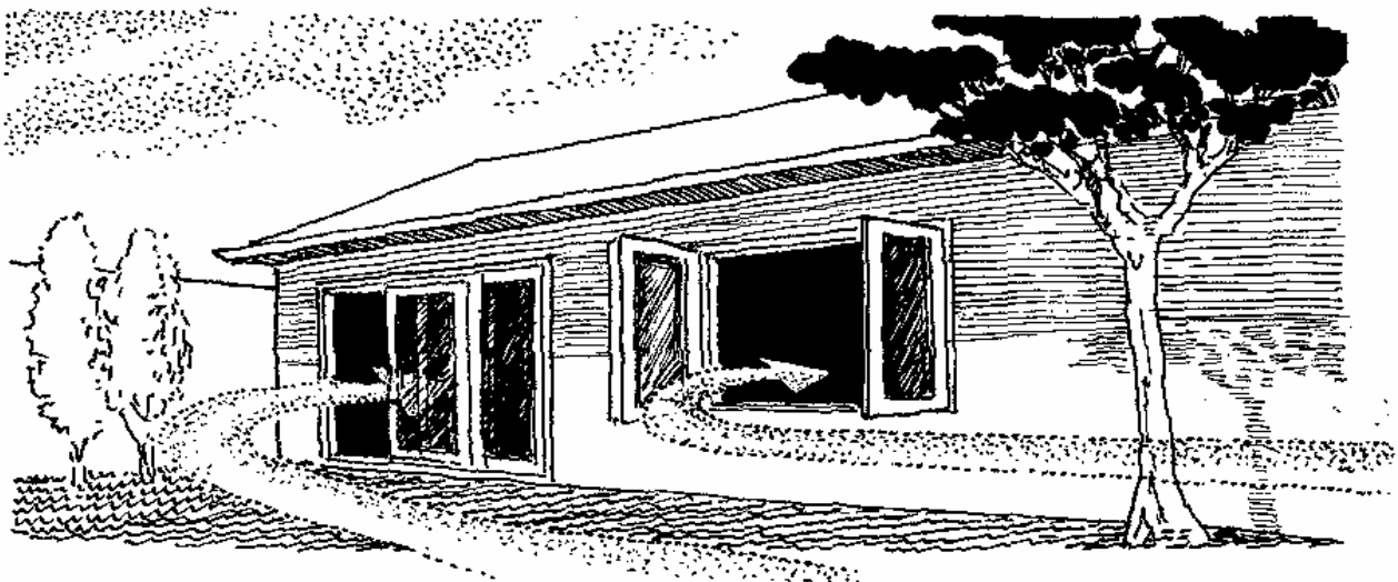
Sliding doors and windows do not help to deflect breeze but external walls or landscape do; casement windows can also help
